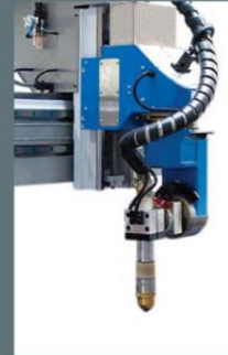
Cutting head moves up and down with Z axis and right and left with X axis.
